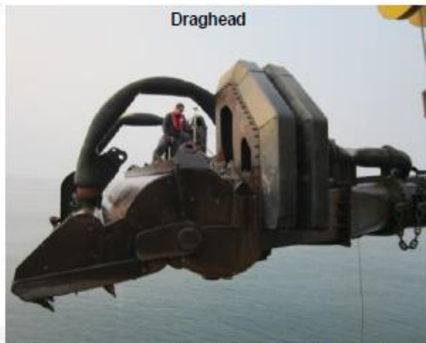
Draghead and suction pipe in operation and detail of a large draghead
